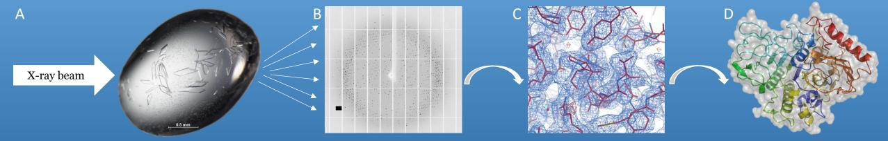
Protein crystals shot with a X-ray beam (A) leave a specific diffraction pattern in form of dark spots on a detector (B). Analysing hundreds of those images from different angles of the crystal results in a density map of the electrons (C), which is used to build the 3D protein structure (D) by incorporating each single amino acid into the electron density map.
