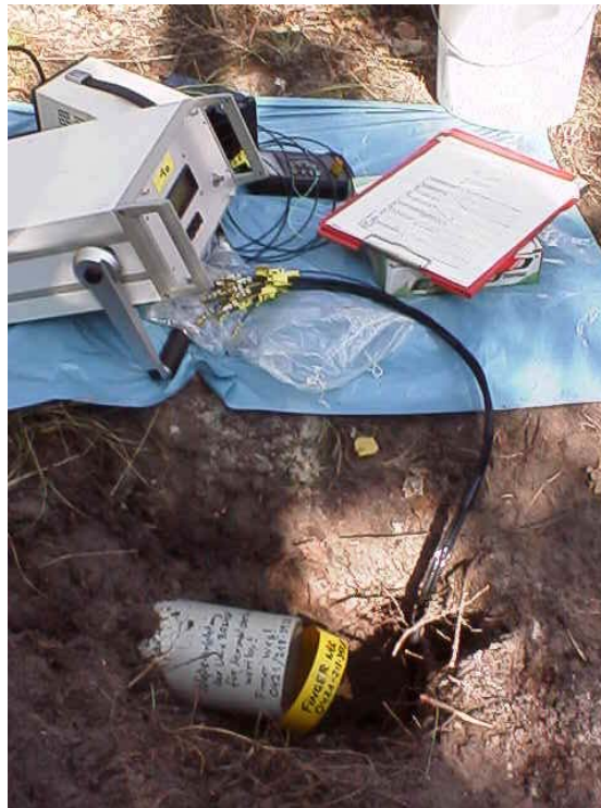
Figure 7: Field situation with a battery-operated MICROX 2 prototype modified for the use with 1 mm POF sensors. 16 optodes (8 oxygen and 8 temperature optodes) were permanently installed in a borehole which was refilled after installation. The instrumental face ends of the fibers are equipped with all metal SMA connectors.
