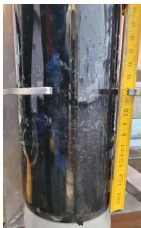
Fig. 3: Sediment core sampled with the multicorer with a high concentration of methane. The corer “bubbled” heavily when brought on deck.
