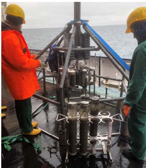
Fig. 3: Several parallel cores of near-seafloor sediments were retrieved with the multicorer. Students Greta and Max are doing the core sub-sampling.
