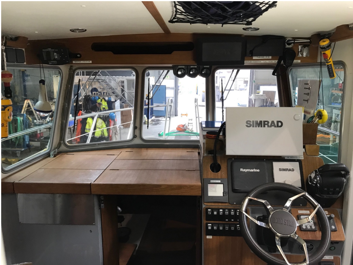
Skipper-console STB, with main 12" SeaChartPlotter, add. Tools (position STB, gliding door).
