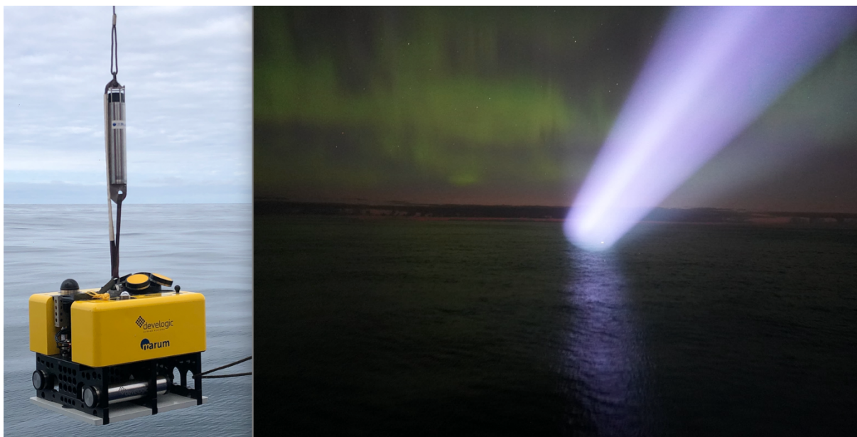
Figure 2 Left: MARUM Seafloor Lander during launch with the Releaser above it. Right: Under colourful Northern Lights skies, the lander surfaces and is followed by the beam of R/V MERIAN until it is safely recovered on board.
