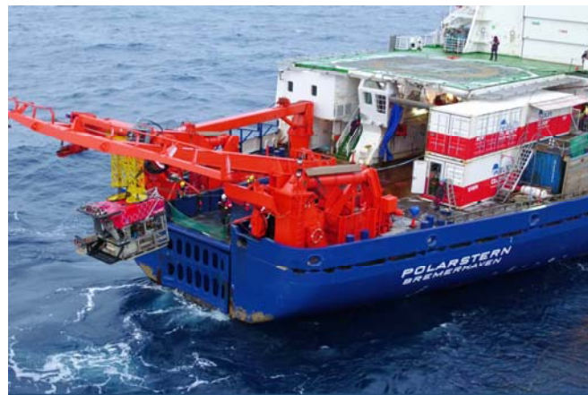
Figure 2: Deployment of MARUM ROV QUEST via the A-frame of RV Polarstern. The aft working deck is almost completely filled by ROV vehicle, winch and containers (© Volker Ratmeyer).
