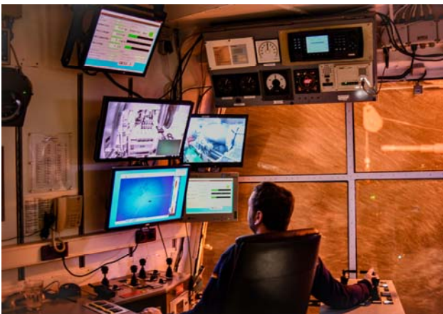
Figure 1: While it is hostile outside during the snow storm, the winch driver sits safe and dry in the winch room of RV Polarstern during equipment deployments (© Vdl).
