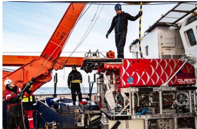
Figure 2: Technical pre-dive checks on MARUM QUEST before the ROV dived to the hydrothermal smokers of the East Scotia Ridge (©vdl).
