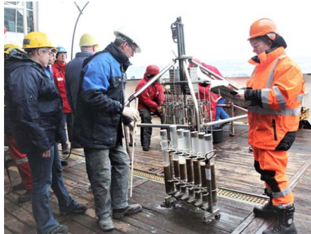
Figure 2: Recovery of full multicorer after arrival of the multicorer on deck of RV Polarstern and distribution of the samples to the different working groups (© Yiting Tseng).
