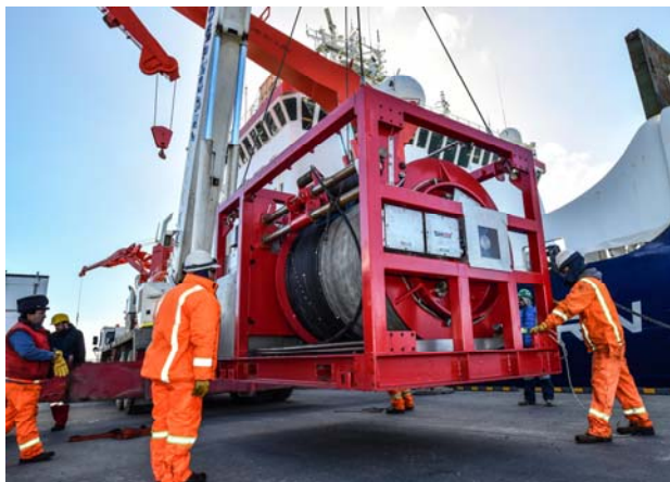
Figure 4: Winch of the MARUM ROV QUEST 4000 just before being loaded onto RV POLARSTERN (© vdl).
