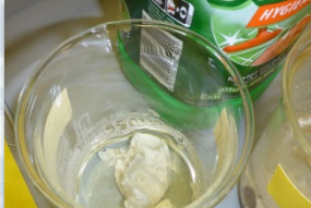
(2) Organic material inside the barnacle removed with NaClO
