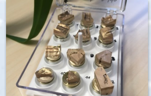
(6) After removal of calcite with HCl - sputter coated with gold
