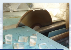
(5) Production of appropriate pieces with a rock saw
