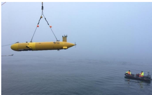
Figure 3: After a long dive, the AUV SEAL 5000 is recovered in the morning. The sea is completely calm here in the Fram Strait near the ice edge and, despite the dense fog, it makes it easier to recover with the rubber boat (@ Gerhard Bohrmann).
