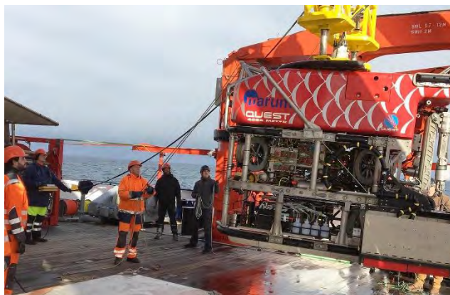
Figure 2: Deploying the MARUM ROV QUEST from the aft deck of the RV MARIA S-MERIAN in the early morning with changing weather conditions (© Gerhard Bohrmann).
