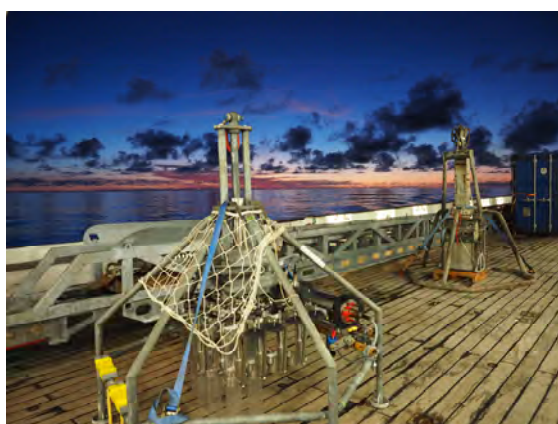
Fig. 4.1 Main sampling tools during the SO-256 expedition. Left: multiple corer, giant box corer, and gravity corer (in the cradle). Right: CTD-rosette water sampler.
